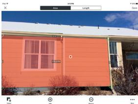
**X** The bump out and the side of the house are on different planes, so you cannot measure the wall if the laser was pointed at the bump out.
