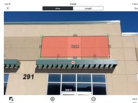
**X** The awning and the wall are not on the same plane, so you cannot measure the wall if the laser was pointed at the awning.
