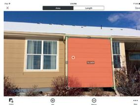
**✓** The bump out is on the same plane that the laser was pointed at (red dot), so measurements will have higher accuracy.
