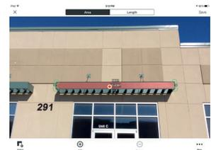
**✓** The awning is on the same plane that the laser was pointed at (red dot), so measurements will have higher accuracy.
